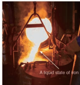
Iron starts melting at about 1 500°C.
