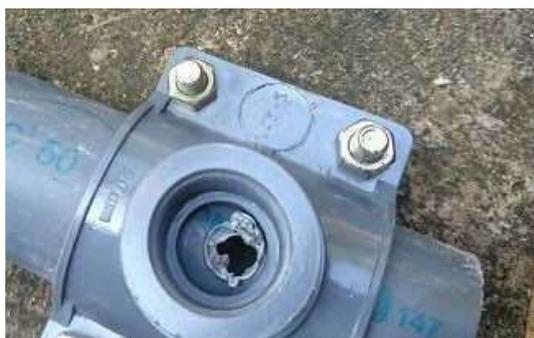
Photo 2 Drilled hole with burr
