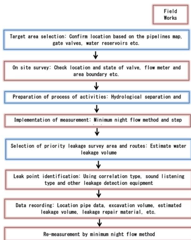
Figure 3 General procedure of leakage control
