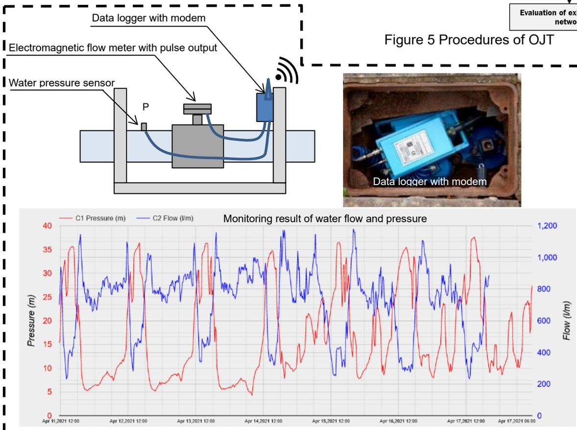
Figure 7 remote monitoring system and monitored water flow and pressure
