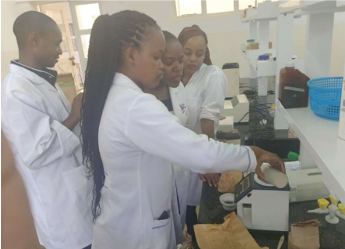
Moisture meter from KETT Electric Laboratory Co. Ltd in use at JKUAT
