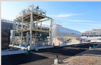
Methanation Using CO 2 Emitted by Waste Incineration
