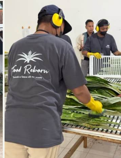
Leaves are placed on a conveyor belt and con- tinuously fed into the fi- ber extractor.
