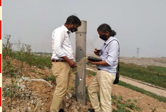
Gas monitoring at landfill site
