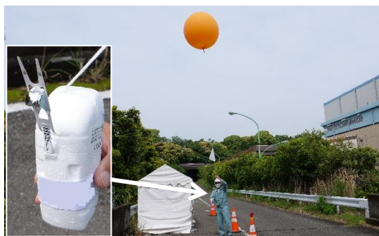
Photo 1-13 Balloon Release for Upper-level Meteorological Survey*
