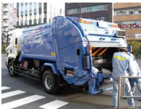
Photo 4-5 Waste Collection by Compactor
