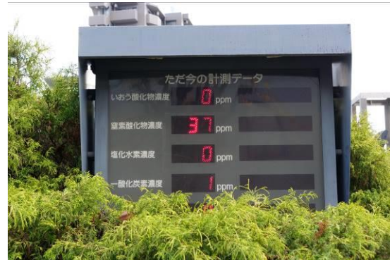
Photo 4-53 Disclosure of Exhaust Gas Status at Shibuya Incineration Plant
