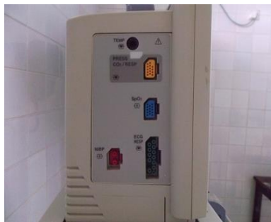
Connection of Blood Pressure, ECG and Pulse Oximeter
