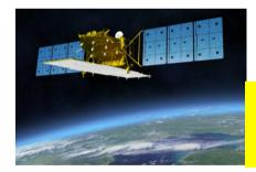
ALOS2 (2014~) also has scan SAR (L-band) sensor which can detect forest change under cloud.
