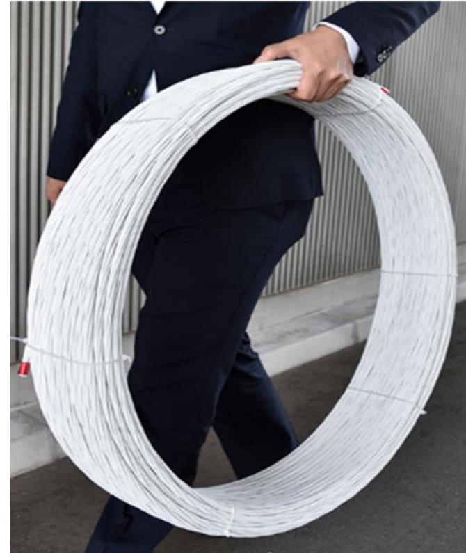
Thermoplastic CFRP roll ,160 meters long, weighs 12 kg!
