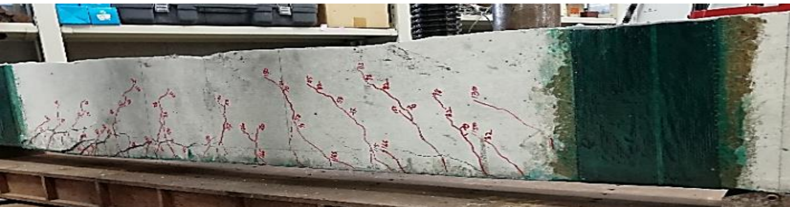
HS8F2A Failure modes=CS Crack nos. =25
