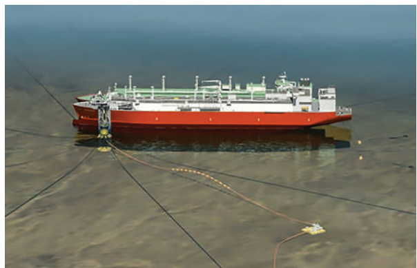
Diagram showing operation of Moheshkhali Floating LNG Storage and Regasification Unit. (Photo: JICA)
