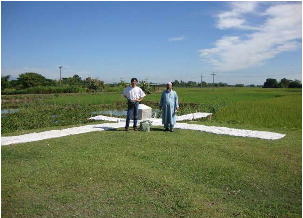
In front of a sign (a white bag filled with sand) to measure the position on aerial photographs (Photo: Bokuro Urabe)
