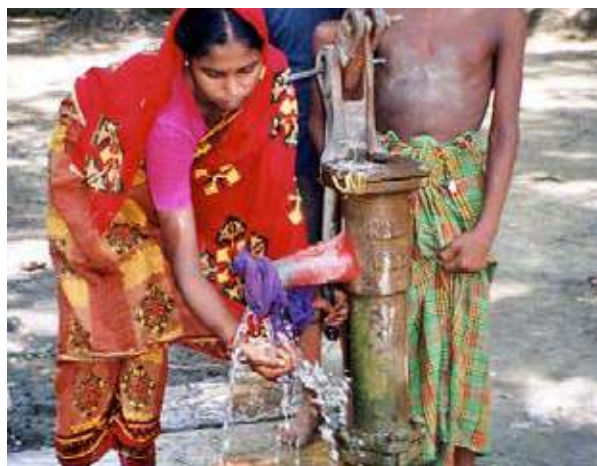
Arsenic contaminated tube well is colored in red after the testing by field kit (Photo: Asia Arsenic Network)
