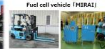
Fuel cell forklift & simple hydrogen filling machine
