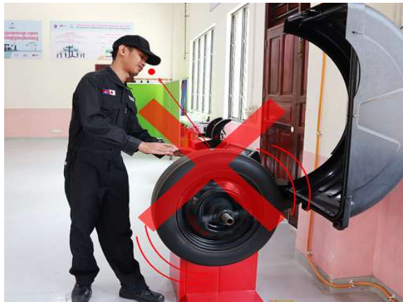
A small pebble flew out while the wheel balancer was rotating.
