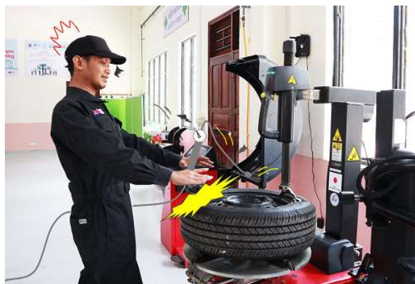
Tire burst while being inflated.
