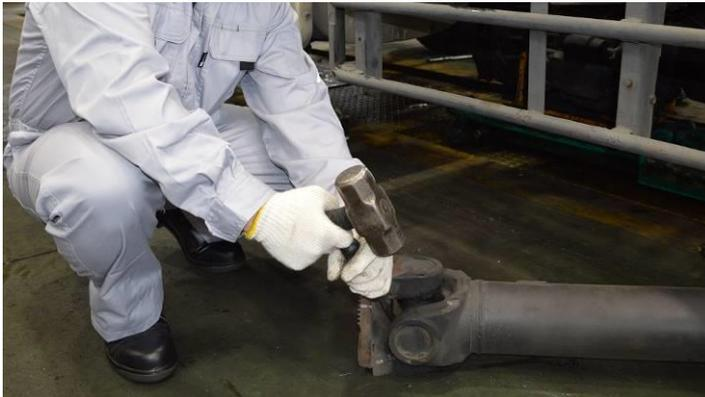
The drive shaft of a large tractor truck was placed on a dolly, and the spider was replaced. In order to remove the bearing, the worker hit the head of the bar with a hammer, but he accidentally hit his right index finger.
