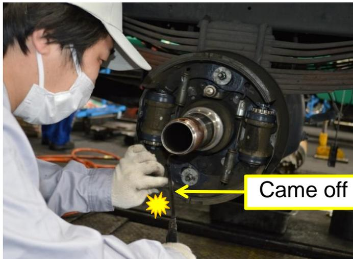
When installing the brake shoe after overhaul of the wheel cylinder, the return spring did not hook on properly, and the worker tried to fit it forcefully. As a result, the spring hook tool came off, and the worker hit their left hand hard against the brake shoe, resulting in injury.
