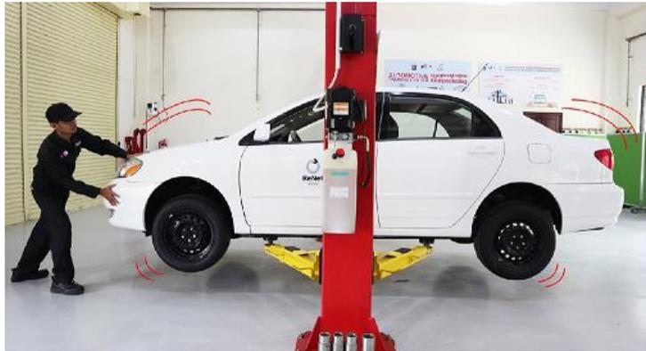
Check the stability of the vehicle with it slightly raised.
