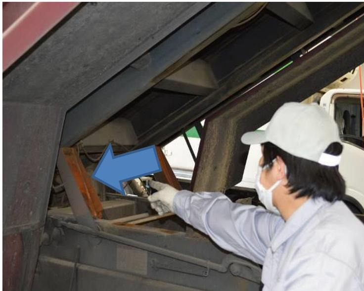
If absolutely necessary to work underneath the vessel, be sure to insert a "stopper" between the vessel and frame to prevent the vessel from falling.
