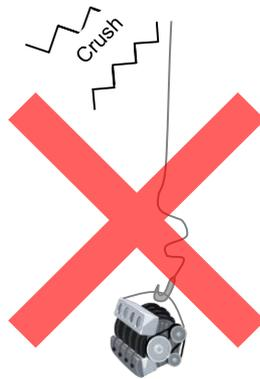
There is a risk of gear damage if parts are hoisted with chain slack.
