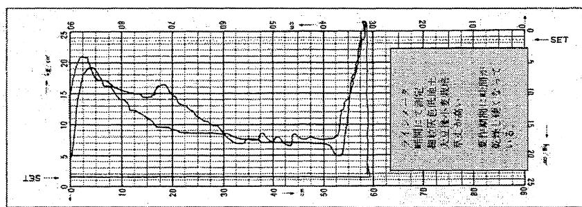
Fig. II -4-2 Sample Data of Penetrometer Profile
