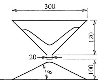
Fig. I -2-2 Angle of Repose
