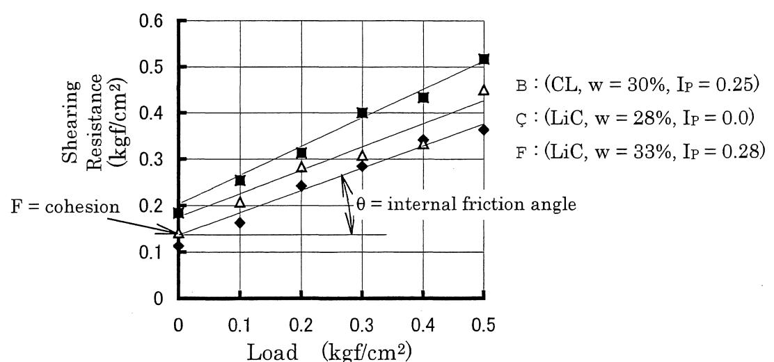
Fig. II -4-5 Relation between vertical load and Shearing Resistance
