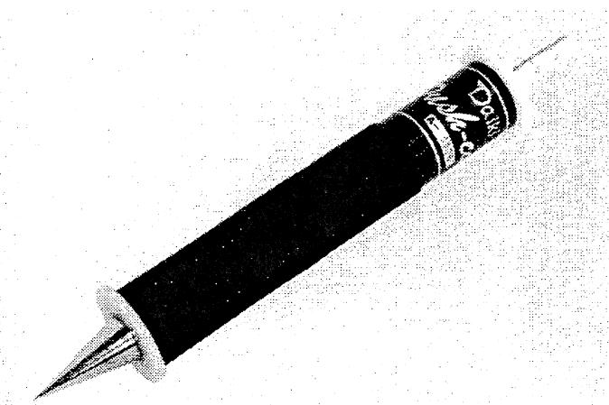
Fig. II -4-3 Soil Hardness Meter , "Push-Cone"
