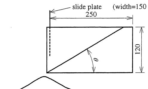
Fig. I -2-3 Angle of Repose
