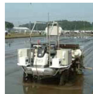
Self-running rice transplanter using GPS
