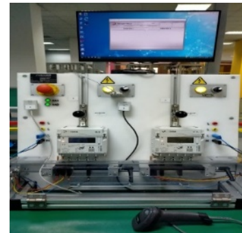
Smart Meters Factory Acceptance Test
