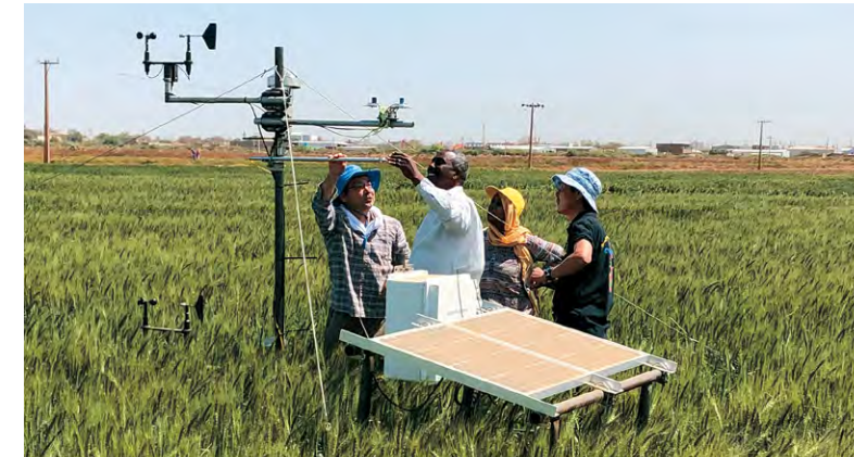
A weather monitoring station installed near the experimental farmland checks the impact of air temperature on wheat cultivation.
