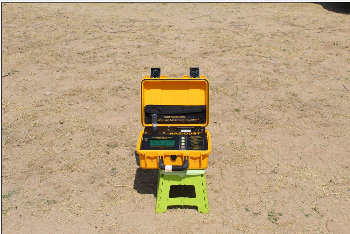
Figure 4-8: Particulate matter measuring instrument used.
