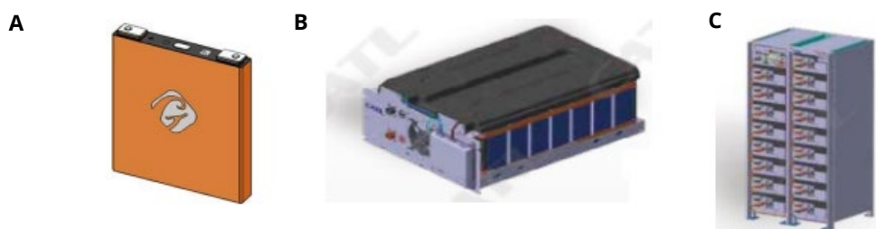
Figure 19: A: Battery cell (175×27×200mm), B: Battery Pack (contains 40 battery cells), C: Battery Cluster (contains 18 battery packs).
