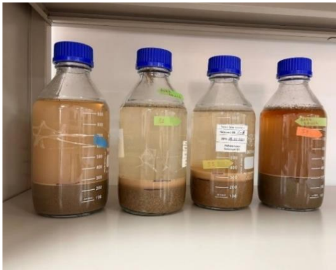
Figure 2: Estimation of soil texture by Bouyoucos method
