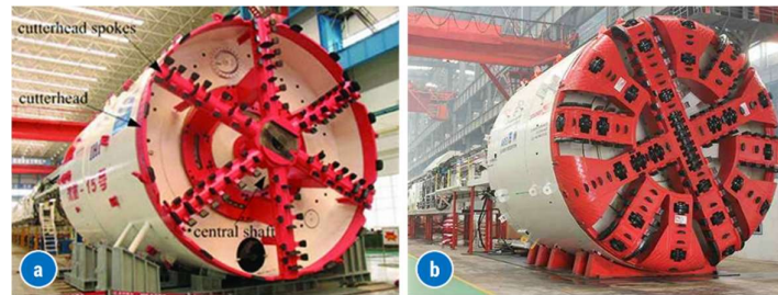
Figure 2.17. TBM cutterhead a) spoke type, b) plate type
