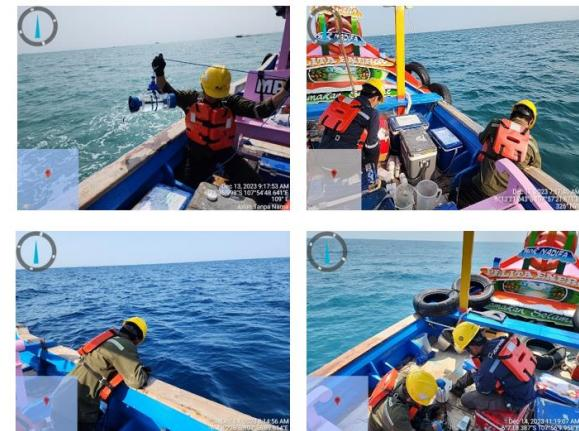
Sea water quality sampling with van dorn tube and indirect measurement of TSS using turbidity meter.
