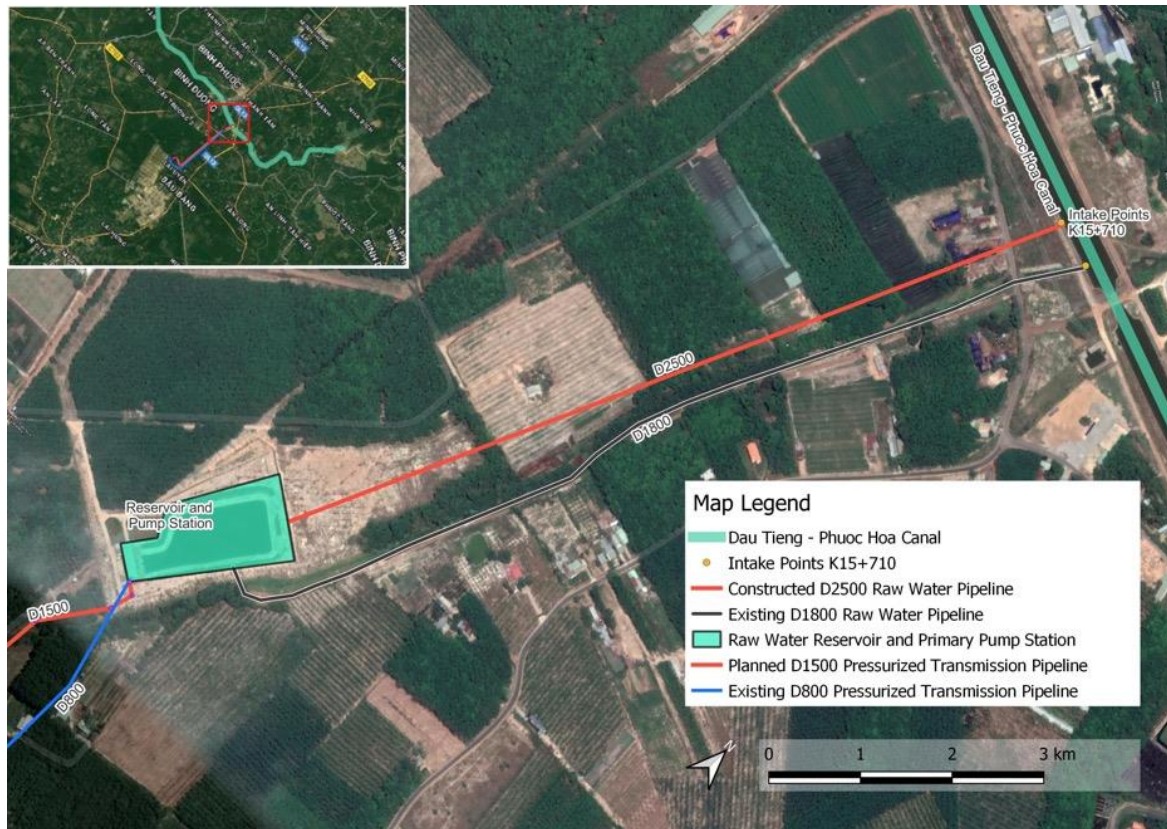
Figure 4-2: Locations of Intake Point, pipelines and pumping station
