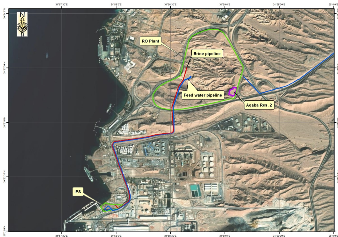
Figure 2-4: Brine Discharge Line from SWRO to IPS
