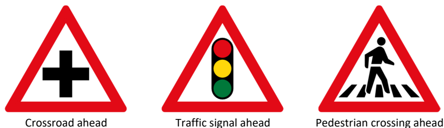
Figure 4.3.6 Example of Warning Signs Installed Near Intersections
