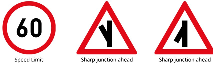
Figure 4.3.4 Example of Regulatory and Warning Signs Installed Near Merge/Diverge Nose
