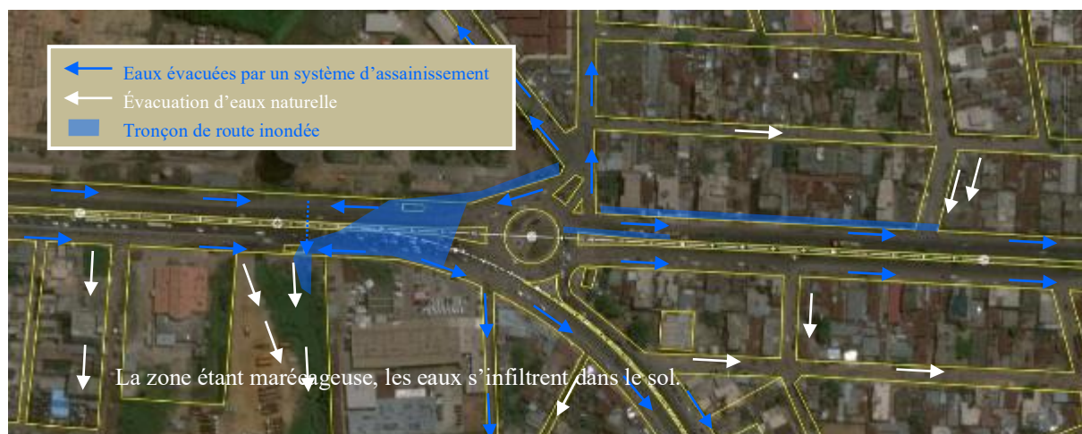
Figure 3: Section of road flooded and direction of water flow
