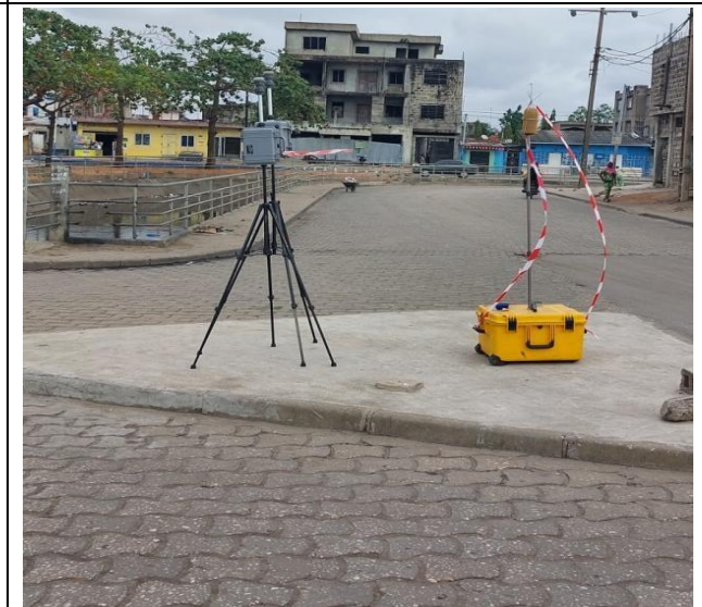
Photo 8: Dust and noise monitoring at the water channel
