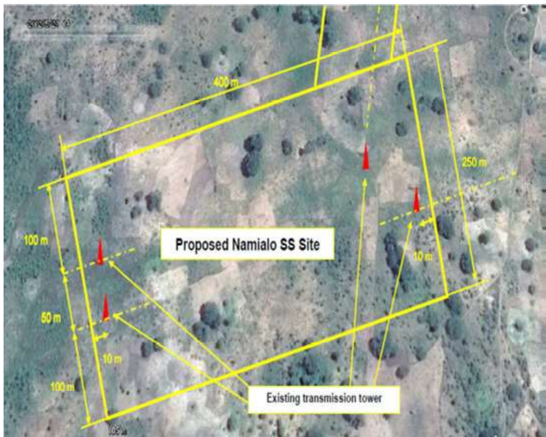
Figure 2: Layout of Namialo Substation Site
