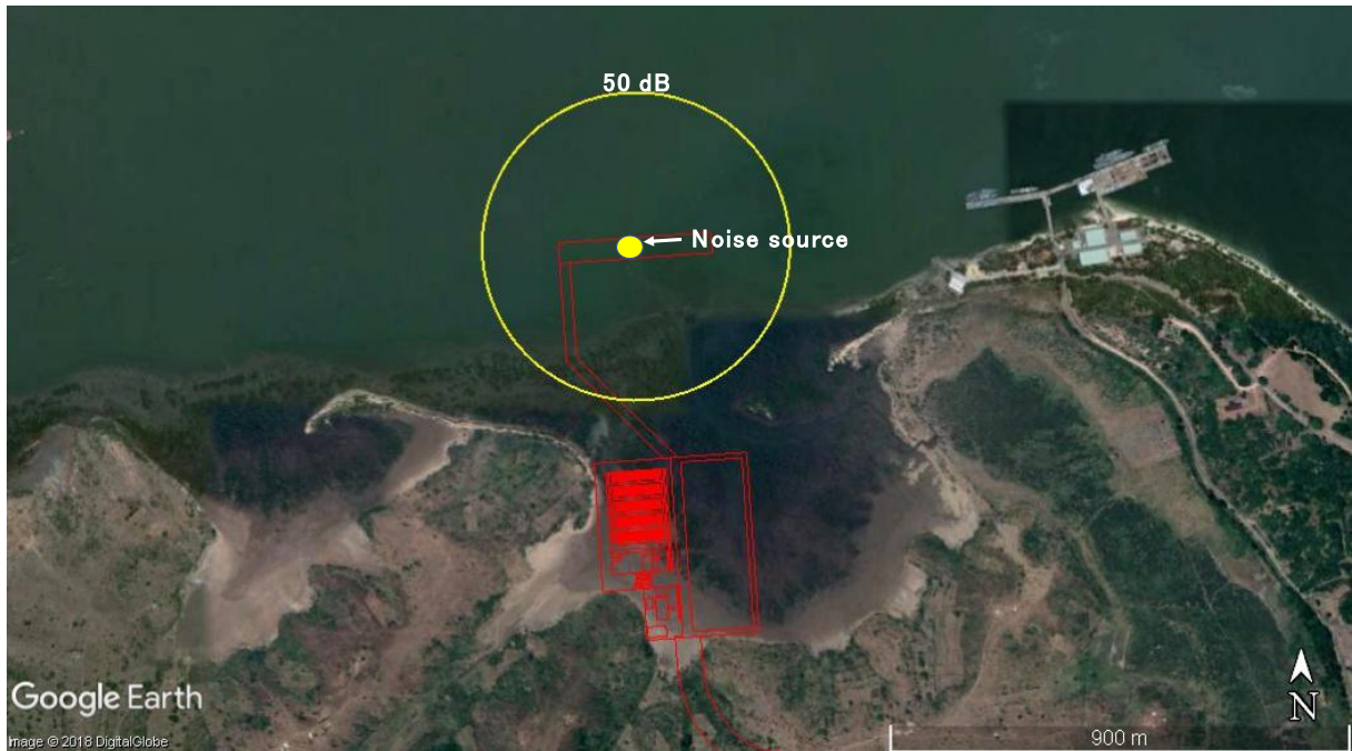
Figure 4.5.1: Predicted noise attenuation from pile-driving works
