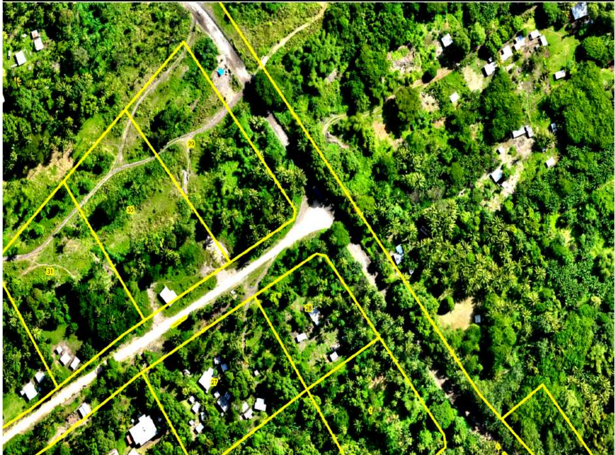
Figure 13.7-14 Drone Ground Control Point Land Boundary Map, 20m Road RoW over the Ranguna section of the road
