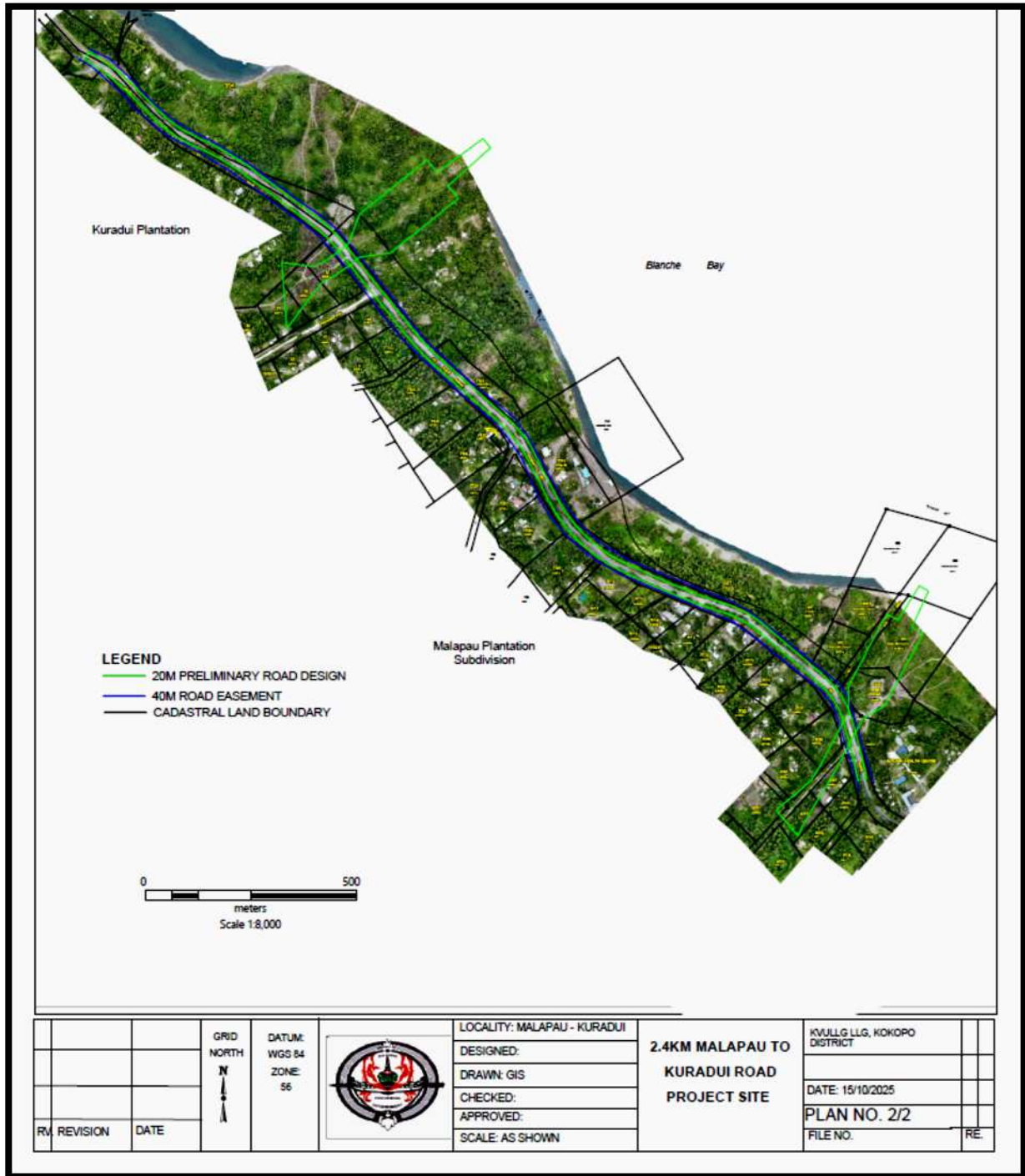
Figure 13.7-10 Drone Ground Control Point Land Boundary Map, 20m Road RoW from Butuwin to Kuradui, the 2.4km road corridor.
