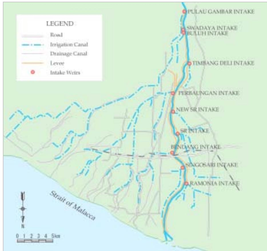
All irrigation facilities and flood control structures (levees) illustrated in the map were constructed under the original project.
