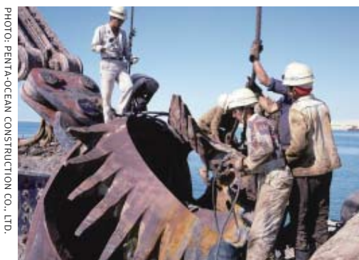
Workers replacing a 3 m diameter cutter blade, which attaches to the end of the ship's rudder.
