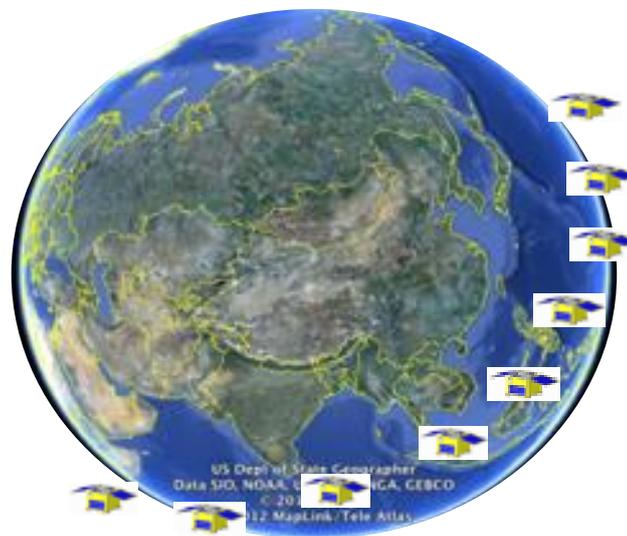
Fig. 6. Equator Orbiter Micro-Satellite Network. As microsatellite in Equator Orbiter observe several times a day, spots scene in cloud free space can synthesize as one belt scene even in optical sensor
