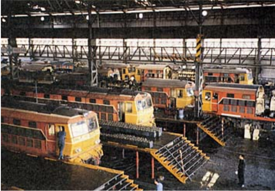
Bangsue depot Periodical Inspection Scenery Light inspection is conducted in front lines, and more precise inspection conducted in profound lines. Railcars in this photo are the same type as ones procured by Project for State Railway of Thailand
