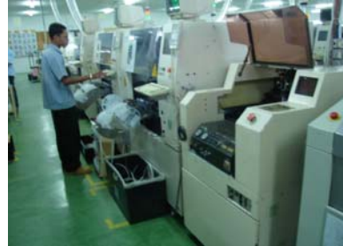
Fig. 8. Electronic circuit board manufacturing equipment purchased with a sub-loan from the project
