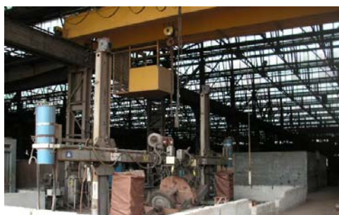
Fig. 1 Railroad Car Workshop in Sekondi (Tire Welding Machine)
