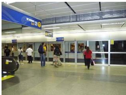
Figure 2: Door shields installed on platforms
