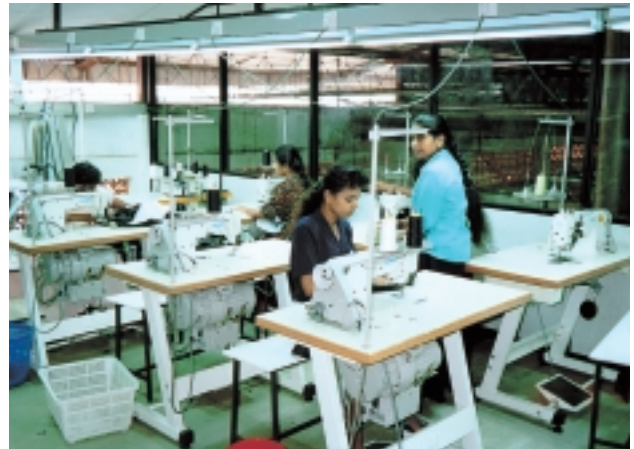
Making samples using sewing machines with thread trimmer
