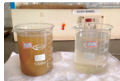
Wastewater at Nagasandra Sewerage Treatment Plant (Left: Before treatment, Right: After treatment)
