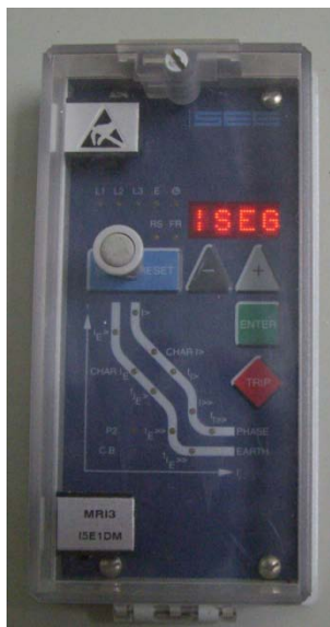
Figure 2.6 Protection Relay and Circuit Breaker after 2000
