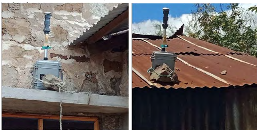
Plate 1: Particulate Matter Measurements (Minivol) and SO x /NO x - May 2018
