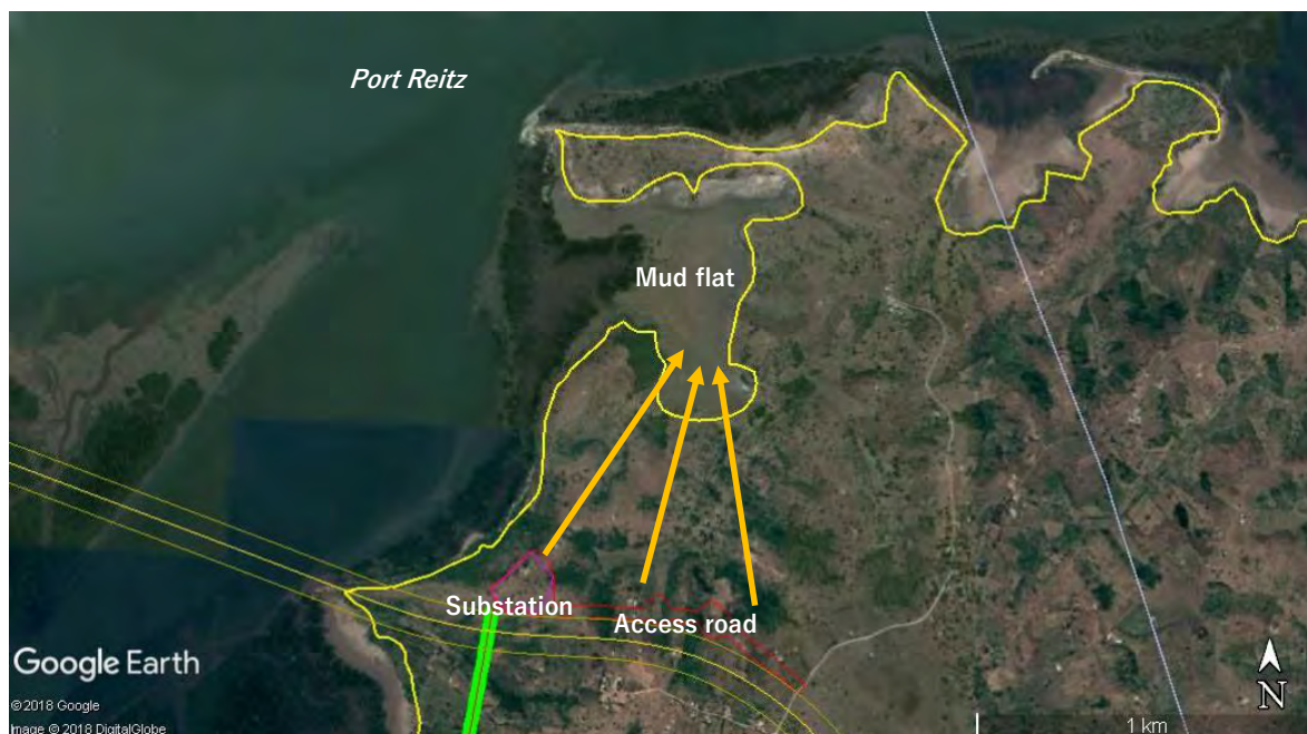
Figure 23: Expected passage of rainwater runoff from substation/access road
