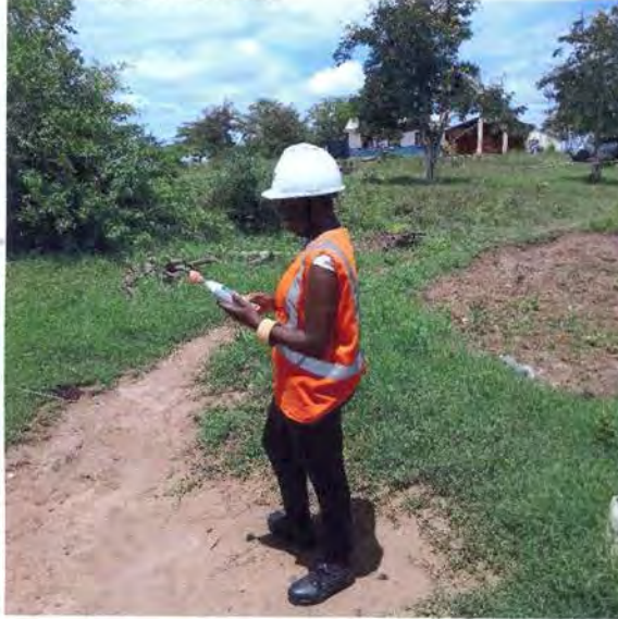
Figure 1 : Field Inspector taking noise measurements using a type II noise meter at substation site
