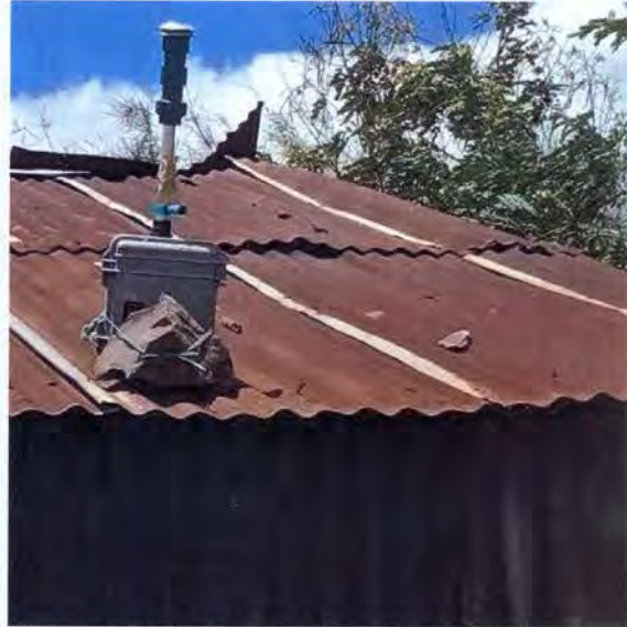
Figure 2 : Particulate matter measurements (Minivol) and SOX/NOX sampling (blue adsorption cartridges) at Pastor Benson's homestead
