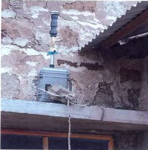
Figure 3:Particulate matter measurements (Minivol) and SOX/NOX sampling (blue adsorption cartridges) at Tsuma Kenga's homestead
