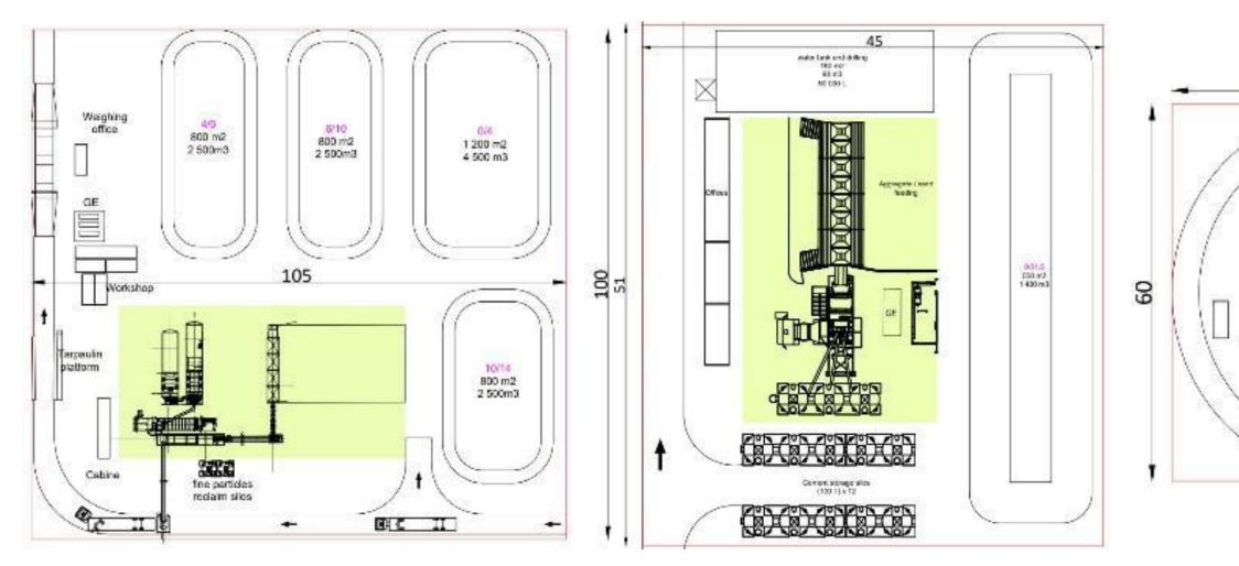
Figure 4-3 Schematic of a Typical Asphalt Production (left image), Mixing (central image) and Emulsion Production (right image) Plants
