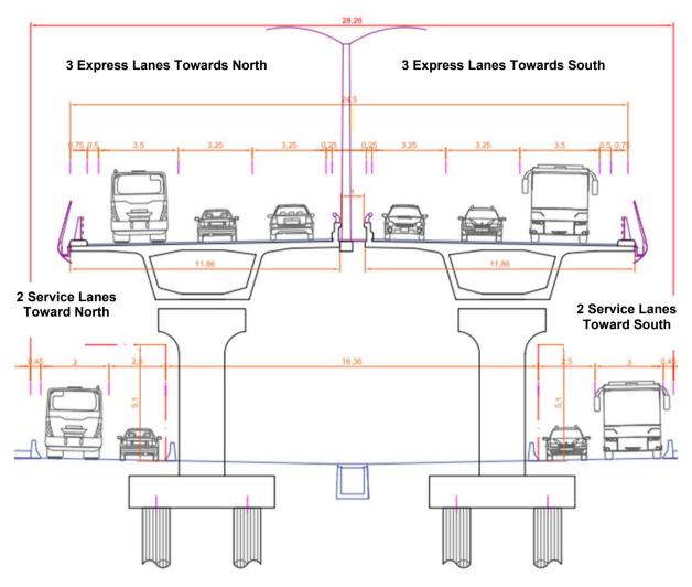
Figure 3-6 Typical Cross Section of a 6-Lanes Flyover
