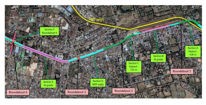
MSE wall section 🛛 Viaduct section 🚽 At grade section 🥥 Roundabout
