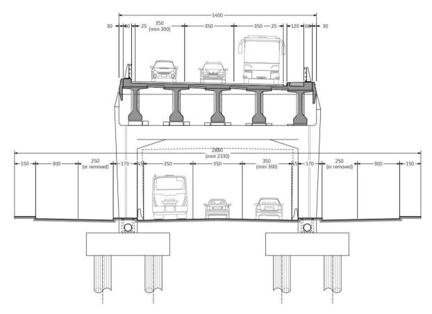
Figure 3-7 Typical Cross Section of a Duplex Type Structure
