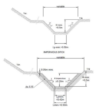
Figure 4-25 Typical Cross Sections of Grassed and Lined Ditches
