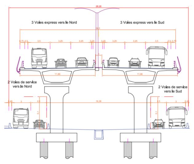
Figure 4-6 Typical Cross-Section of the Flyover
