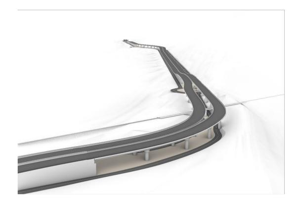
Figure 4-7 3D Representation of the First Flyover Section over Nakuru's 1<sup>st</sup> Roundabout with a view on the at Grade section
