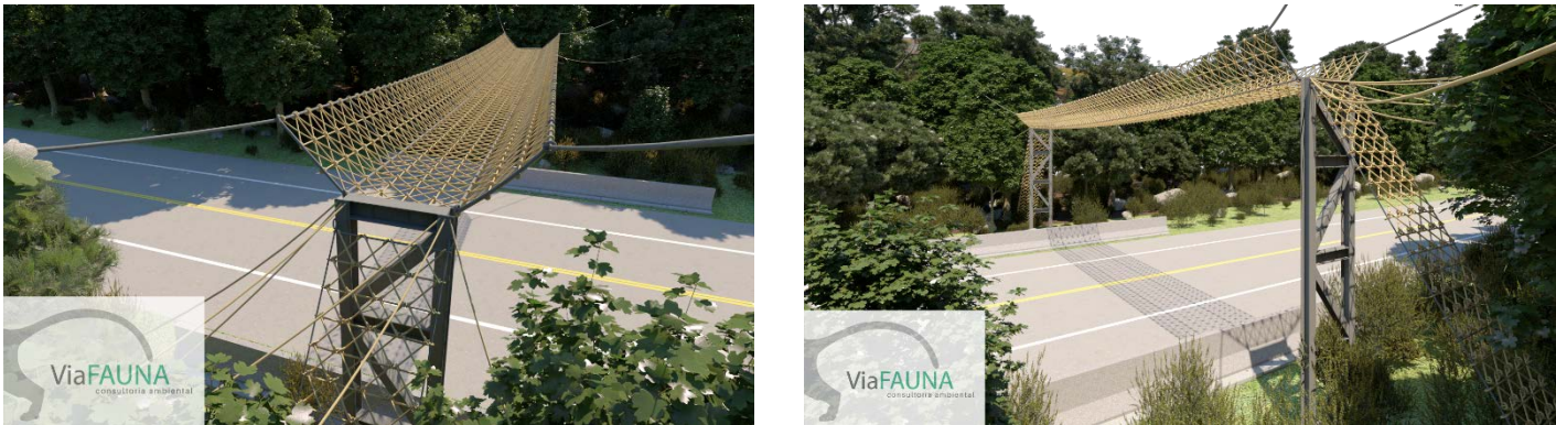
Figure 4.12. Design of canopy bridge being tested for use by primates in South America and proposed for further testing on the A8 and A8South Project. This should be tested against other potential designs to evaluate use and effectiveness. Design by Fernanda Abra, ViaFauna, Brazil.
