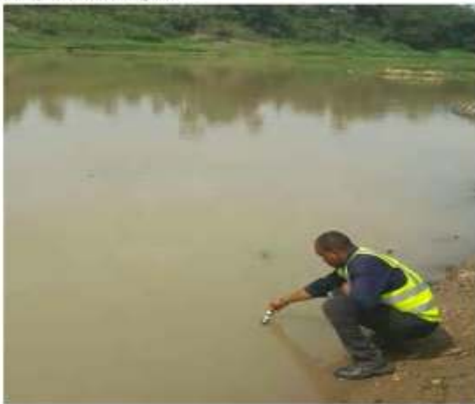
Plate 4.11: Insitu measurement of unstable parameter using Hanna Combo Water Tester HI 98130
