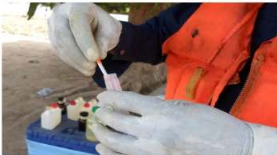
Plate 4.5: In- situ Test for Bateria Species using Watersafe Rapid Bacteria Test Kit
