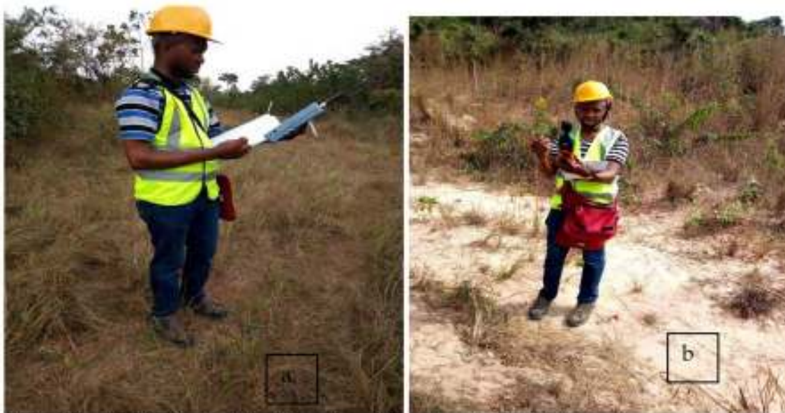
Plate 4.2: EMF (a) and Noise Sampling (b) during the field survey
