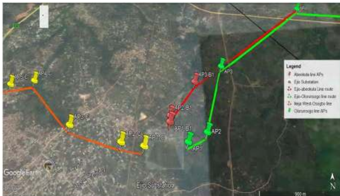
Figure 3.11: The three transmission line route from Ejio substation
