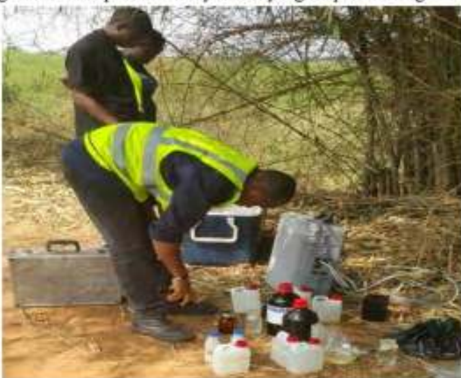
Plate 4.10: Preservation of Surface Water Sample with high grade analytical Preservatives
