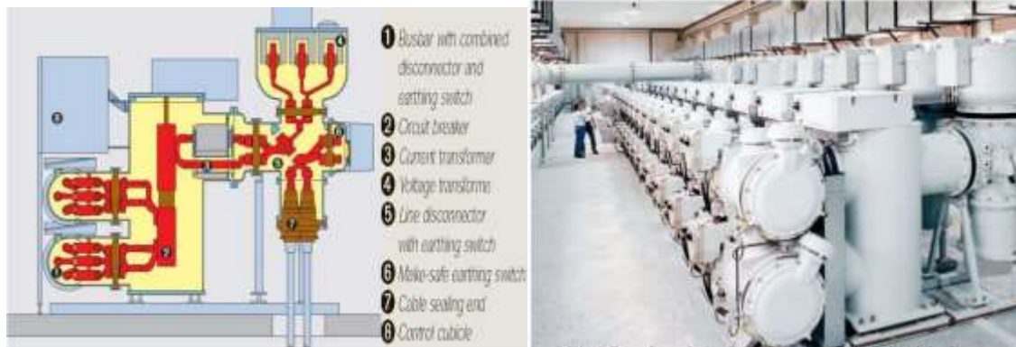
Figure 2.2 Gas Insulated Substation with Double Bus Arrangement
