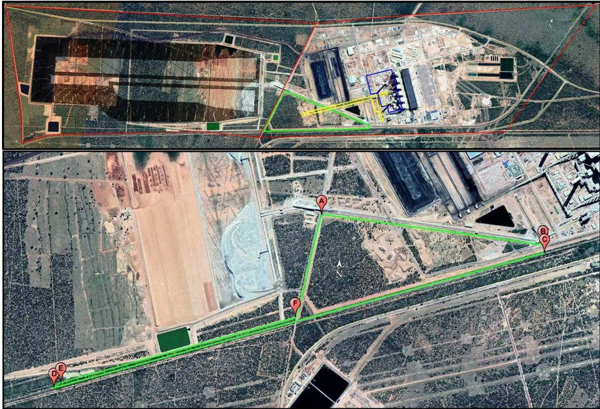
**Figure 6-3: Proposed railway yard development area, including limestone and gypsum handling and associated infrastructure (green outline) between the MPS and existing ADF**
