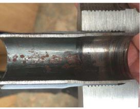
Corrosion of a carbon steel tube.
