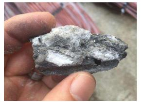
Fly Ash build-up retrieved from the tubes during maintenance.
