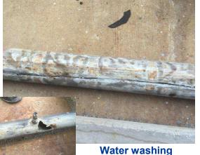
Wear damage of system cracking carbon steel tube. due to corrosion.
