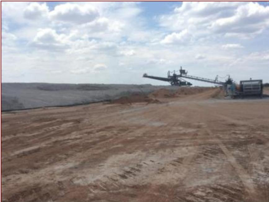
*Figure 45- Machine that loads ash onto the facility from conveyor belt*
