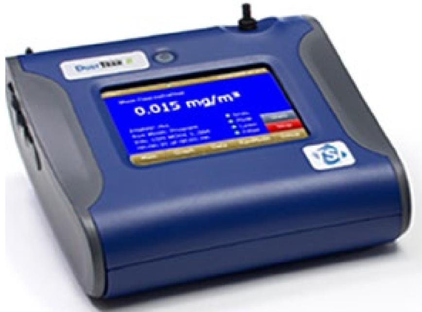
Figure 4-9 Dust Track II 8530 used for dust sampling
