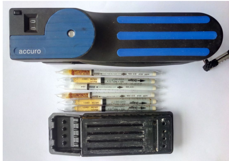
Figure 4-11 Dräger gas detection pump and Tubes
