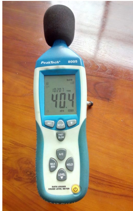
Figure 4-12 Peak Tech 8005 sound level meter
