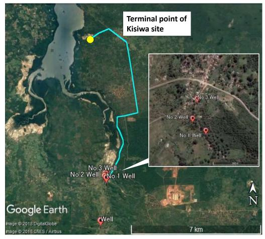
**Figure 2-33 Proposed Water Supply Pipeline Route** Source: JICA Study Team, 2018
