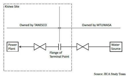
Figure 2-10 Water Pipeline Terminal Point
