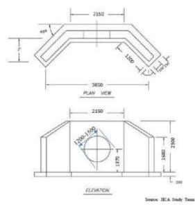
Figure 2-19 Planned Culvert Design Source: JICA study team, 2018
