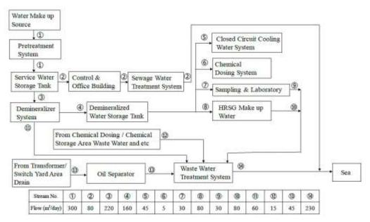
Figure 2-14 Water Treatment Flow (Water Balance)
