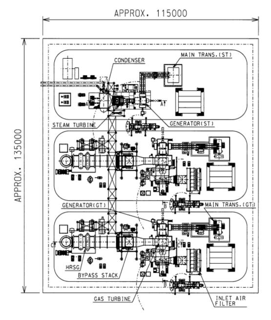
Figure 2-6 Typical GTCC Layout of Heavy Duty GT with Seawater Cooling System
