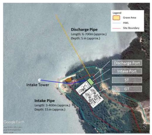
*Figure 2-16 Conceptual Layout of Intake and Discharge Streams Source: JICA Study Team, 2018*
