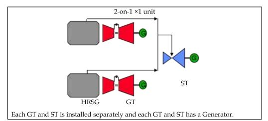
Figure 2-8 Schematic Diagrams of multi-shaft 2-on-1 GTCC Source: JICA Study Team, 2018
