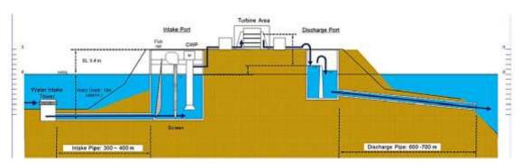
*Figure 2-15 Cross-section of Intake and Discharge Structures Source: JICA Survey Team, 2018*
