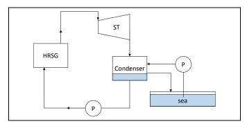
Figure 2-9 Schematic System Diagrams of ST Cooling Type Source: JICA Study Team, 2018
