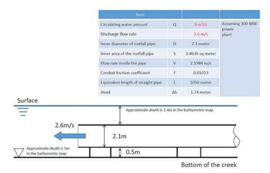
*Figure 6-10 Outfall Configuration for 300MW Case* Source: JICA Study Team, 2018
