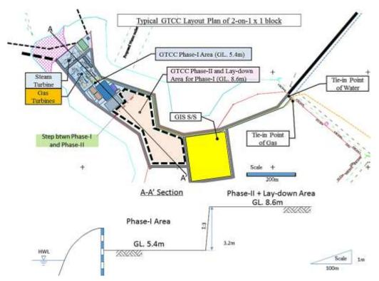
*Figure 2-30 Layout and Sectional View of Project Phase I and Phase II Areas Source: JICA Study Team, 2018*
