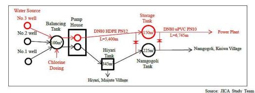
*Figure 2-11 Proposed Water Supply System for the Mtwara GTCC Power Plant (black: existing, red: proposed)*
