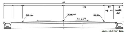
Figure 2-23 Proposed draft design of Roads with Roadside Ditch
