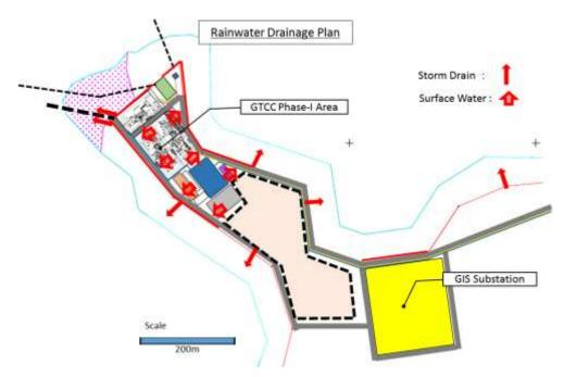
Figure 2-17 Draft Plan of Rainwater Drainage System
