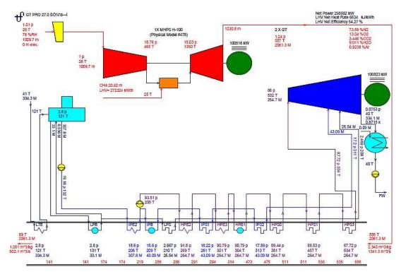
Figure 2-7 Heat Balance Diagram of Heavy Duty GT Source: JICA Study Team, 2018
