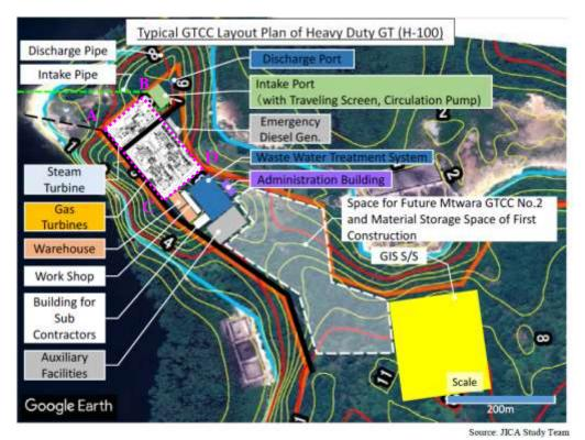
*Figure 2-5 Layout of Project Components Source: JICA Study Team, 2018*
